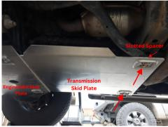
Remove 4 rear bolts from support tubes. Lift OKX Transmission Skid Plate and slide front into position above the Mid Plate. Attach rear of Transmission Skid Plate using supplied **M8x45mm** bolts & washers. Position slotted spacers between the Transmission Skid Plate and tube support tabs.
