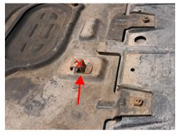
Cut off the small hook and grind any remaining material flush with the surface of the skid plate. Paint any exposed metal to prevent rust.
