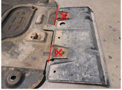
Cut off the 2 rear tabs holding the plastic shield. Trim these flush with the rear edge of the skid plate.
