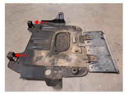
Remove the stock Mid Plate. Retain hardware from the front 2 mounting points for re-use. The Front Skid Plate can remain on the vehicle.
