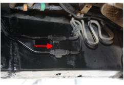
**Driver Side Frame:** Remove M8 bolt securing brake line bracket to frame.
