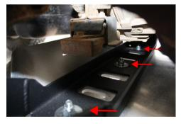
Tighten Nyloc nuts snug. Tighten M8 Bolts to 28ft-lbs.
