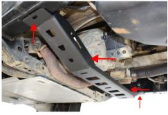
Slide Crossmember forward, and push up flat against the bottom of the frame. Snug M8 bolts to hold Crossmember in position.
