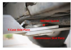
Reinstall the original slotted spacers into the top position as shown. Do not use the new supplied spacers at this time.
