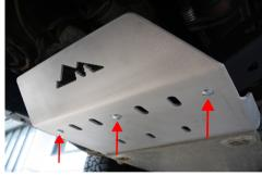
Install (3) supplied 3/8" x 1-1/4" Carriage bolts up through Skid Plate and Crossmember. Secure with large flat washers and Nyloc nuts.
