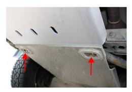
Install supplied *M8x50mm* bolts and washers through Transmission Skid, T-Case Skid, slotted spacers, and into frame. Align T-Case Skid Plate with Transmission Skid Plate and new Crossmember. **Do not tighten yet.**
