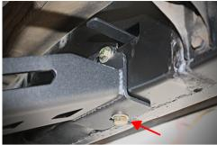
Install supplied *M10x30mm* bolt and washer up through Crossmember and frame, into the Tab Nut. Repeat for opposite side.
