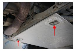
Remove (4) M8x45mm bolts and slotted spacers from rear of Transmission Skid
