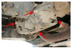
Remove 4 bolts holding factory T-Case Shield on. Remove T-Case Shield.
