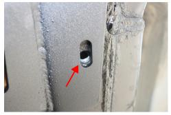
Position the Tab Nuts on each side so the threads can be seen through the crossmember and lower frame holes.
