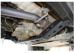
Lift new Crossmember into place. The ends are angled in toward the front to match the frame. **Driver Side:** The Crossmember should be behind the brake line bracket
