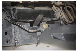
The Tab Nuts should be sitting flat inside the frame, with no dirt or sand in the way. The Tab end will be sticking out of the frame access hole.
