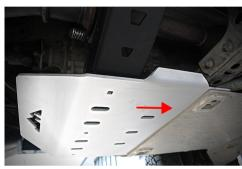
Position T-Case Skid Plate above Transmission Skid Plate. Loosen the front Transmission Skid Plate bolts if needed.
