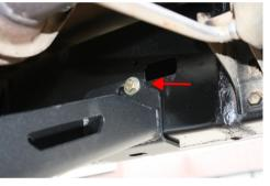
**Passenger Side:** Install supplied *M8x30mm* bolt with washer through Crossmember and into factory frame hole. Do not tighten yet.
