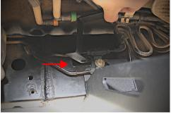
Insert Driver Side Tab Nut into frame access hole, with the nut position toward the front of the truck. Repeat for Passenger Side Tab Nut. **Do not lose Tab Nuts inside frame.**
