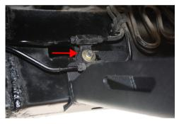
**Driver Side:** Install supplied *M8x30mm* bolt with washer through brake line bracket and Crossmember, into factory frame hole. Do not tighten yet.
