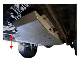
Level the skid plate left to right, and tighten front inner bracket. repeat for the rear brackets. Re-check tank clearance around perimeter & brackets.
