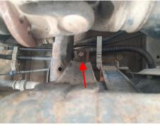
Next, remove the rear inner bolt located above the rear end of the driveshaft.
