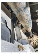
Loosely install the medium bracket at the front inside location.
