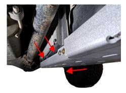
With all brackets loosely in place, adjust the skid plate towards the driveshaft and check for clearance along the tank inner side. Check tank clearance around entire perimeter. Tighten 3 front outer frame bolts.
