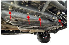
Remove the remaining 4 bolts along the frame, and lower the factory shield away from the vehicle.
