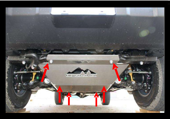
4. Install OKX Engine Skid using 4 factory bolts, and supplied M8x35mm bolts, washers & 3/8" spacers.
