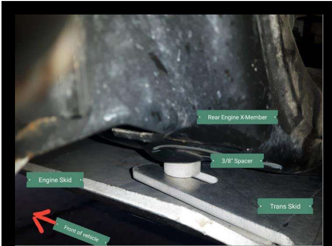
When installing OKX Transmission Skid, loosen rear Engine Skid bolts and slide Trans Skid between x-member and Engine Skid. Li 3/8" spacer up to x-member.
