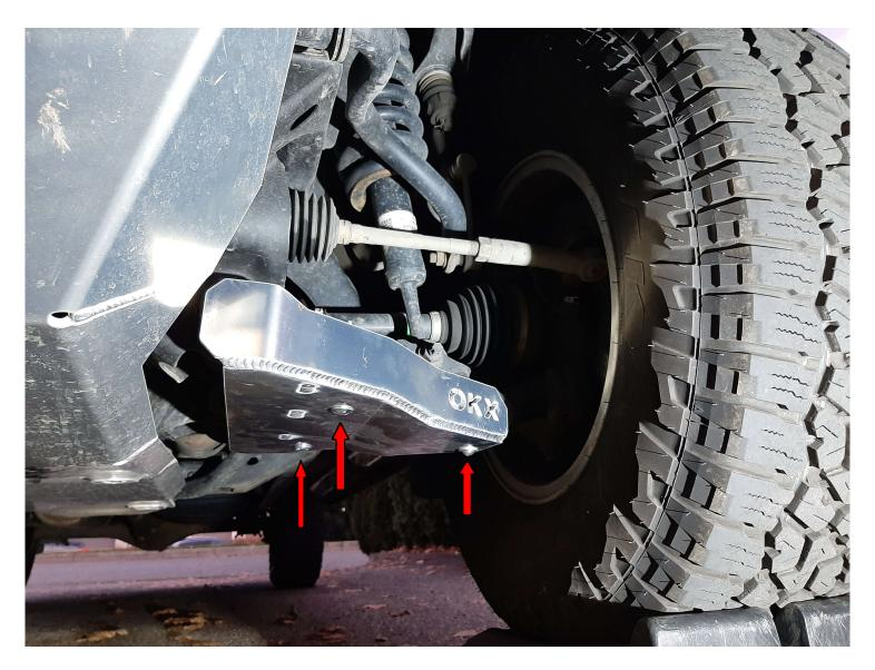
Install Lower Control Arm Skids using supplied hardware. 3/8"x 3.5" Carriage Bolt at the rear. 3/8"x 3" Carriage Bolt at the front. 5/16"x 2.5" Buttonhead bolt w/washer at the outer hole.
