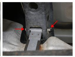
Remove clip and mounting pin from tank strap - located above driveshaft. Save hardware. Transfer rubber tank isolator to new strap. Reinstall new strap using original hardware. Repeat steps for rear tank strap. **Torque Strap Bolts to 46ft-lbs**
