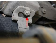
Remove tank strap bolt located on driver side frame rail. Save hardware.
