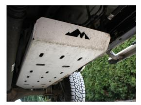
Adjust Gas Tank Shield so there is even clearance between the tank and Shield on both sides. Ensure clearance along frame. **Tighten hardware to 18ft-lbs.**
