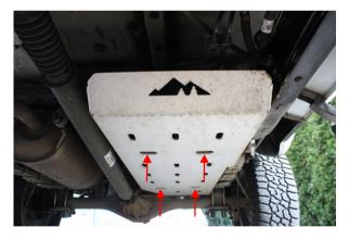
Tank Shield Installation OFF-ROAD models- Support factory tank shield and remove 4 bolts holding shield in place. Remove factory tank shield. Lift OKX Gas Tank Shield into position, locating 4 tank strap studs into slotted mounting points.
