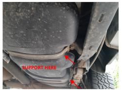
Tank Strap Replacement (Non OFF-ROAD models only) Install easiest with 1/4 tank or less. Support tank near front strap with a floor jack. Only remove and replace 1 strap at a time.
