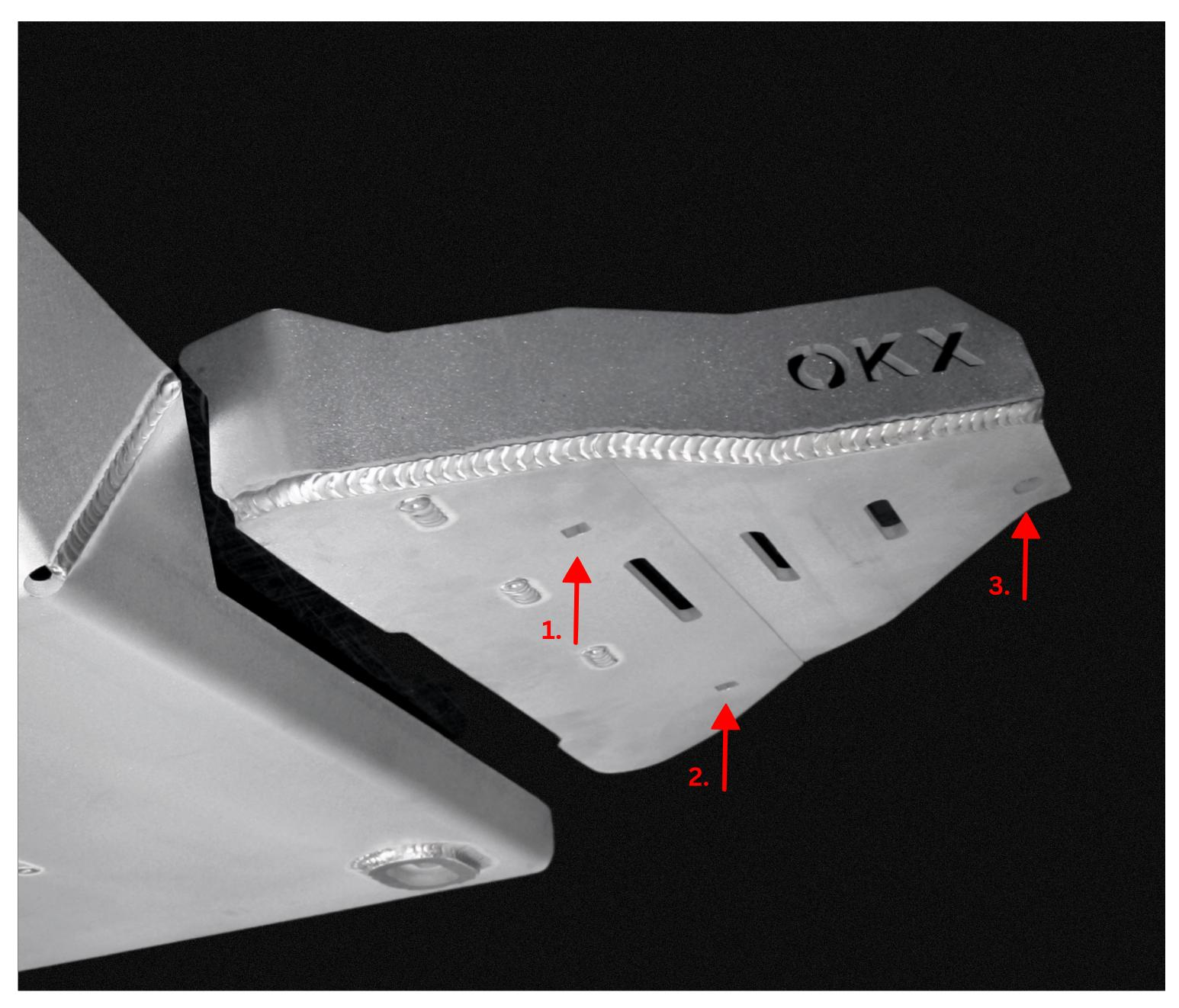
Any factory hole plugs will need to be removed before installation.
