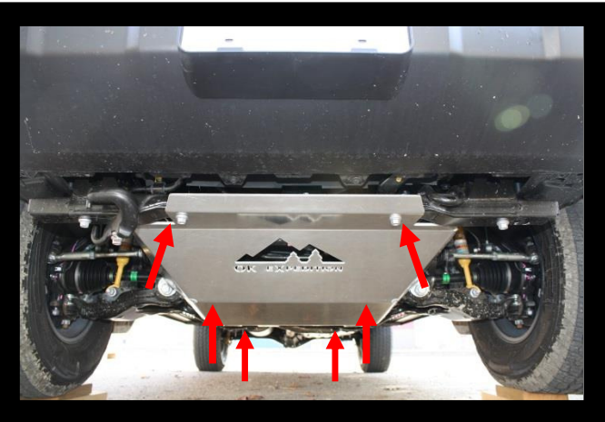
4. Install Engine Skid using 4 M12 factory bolts, and supplied M8x35mm bolts, washers & 3/8" spacers.
