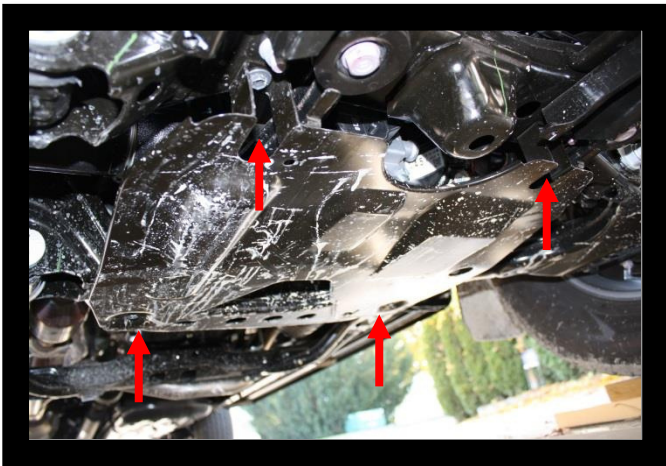
2. Remove 4 bolts and rear Engine Skid (if equipped).
