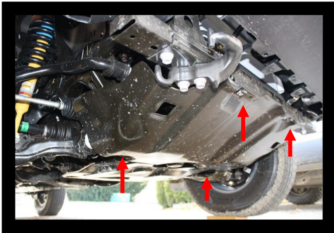
Remove 4 bolts and factory front Skidplate.
