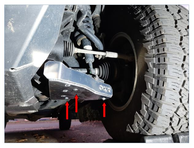
Install Lower Control Arm Skids using supplied hardware.
